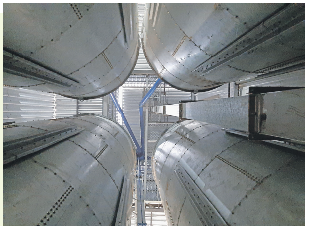
Acquisition and installation of 4 silos with a total storage capacity of 100 tons of black pepper.
