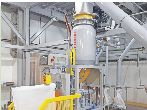
Acquisition and installation of a semi-automatic packaging machine with bagging capacity of 8 tons per hour.
